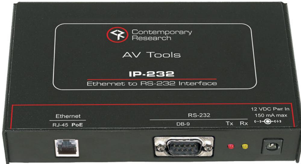
The IP-232 extends Ethernet control to CR's 232-series TV tuners, video projectors, displays, and other RS-232 controlled equipment. The IP-232 is PoE compliant, accepting power through the LAN in either A or B modes. The unit is fully programmable, and includes switch settings to aid in installation.
