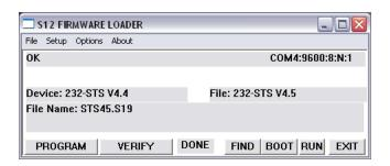
This S12 firmware loader (S12L152.EXE) is included with the ICC2-ATSC 4/4S Firmware Pack. The ZIP folder includes the S12 and HD Load firmware installers.
