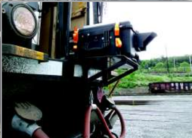
Two views of the custom camera case mounted on the nose of the locomotive. The solar panel on the top maintains the batteries during wireless camera use.
