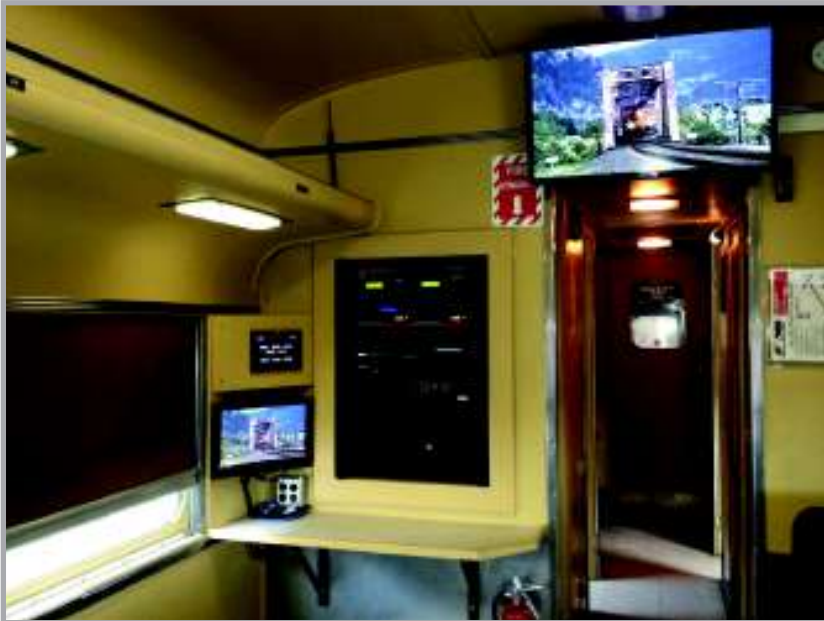
This is the operator control space for the AV systems in NS-28, and also shows one of the seven 32-inch displays in the car.
