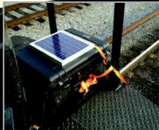
Two views of the custom camera case mounted on the nose of the locomotive. The solar panel on the top maintains the batteries during wireless camera use.
